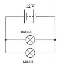
(a) Show that the resistances of bulb A and bulb B are 7.2  $\Omega$  and 28.8  $\Omega$  respectively.
